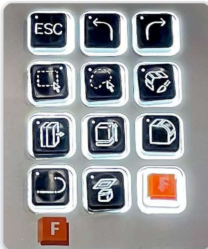
The finished overmolded keycaps complete with engraving
