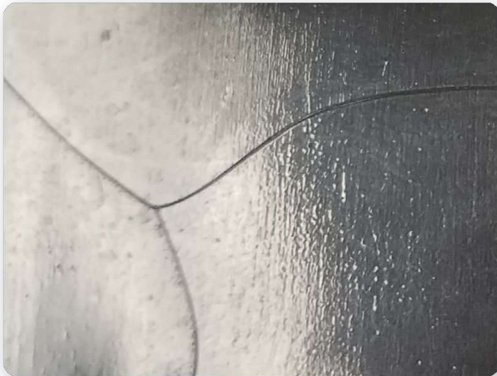
An example of knit lines on a part
